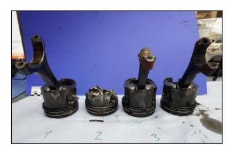
The first conclusions are that the engine stopped operating further to a mechanical break-up of the Nr 2 Piston. Extensive testing on the FADEC installed on the engine were performed. The report is inprogress.
