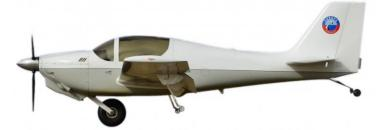
Figure 2 : Europa Classic Monowheel with the flaps and outriggers retracted
