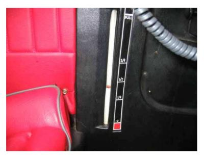
The gauges are accurate on the ground, but in flight their accuracy is reportedly unreliable.
