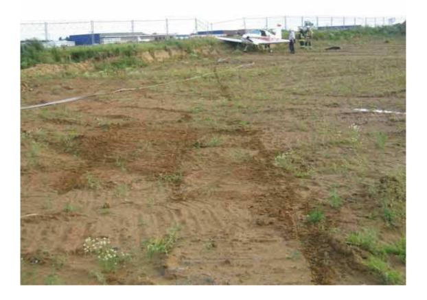
The aircraft touched the ground parallel to the runway, rolled for 60m, then veered towards the embankment slope bordering the airport perimeter.
