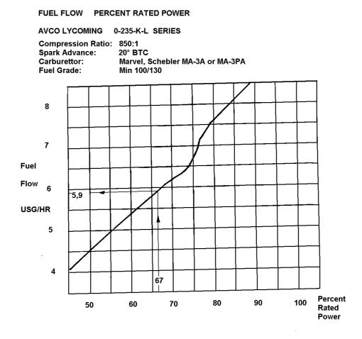
If we combine the Grumman's and the Lycoming's chart, for an engine rating of 2450rpm – altitude 2500ft, the Grumman chart gives 67 percent power.
