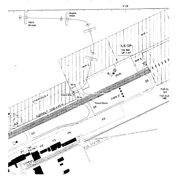
The engine stopped when the aircraft reached the airport zone. The pilot wanted to land the aircraft as soon as possible, and directed the aircraft in a glide dive in the direction of the airport tower. The aircraft never reached the runway, and landed on a construction zone outside the perimeter of the airport. The aircraft touched the ground parallel to the runway, rolled for 60m, then veered towards the embankment slope bordering the airport perimeter.
