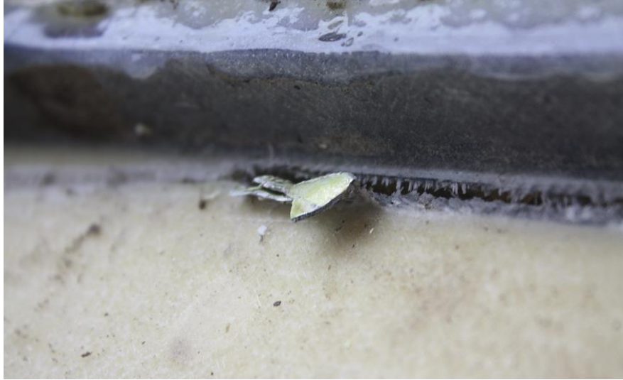
Figure 22: Metallic part in the right wing spar.
