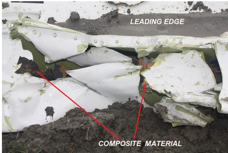
Figure 27: Impact damage on the C172 LH wing leading edge
