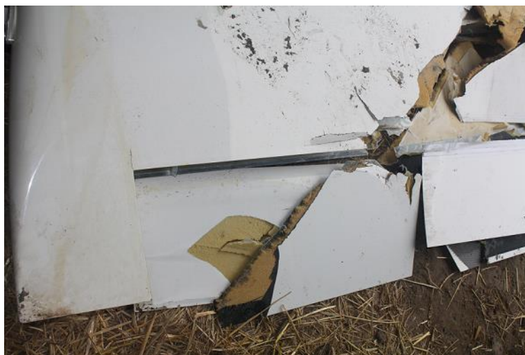
Figure 21: Right wing aileron damage (lower side)
