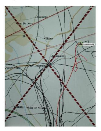
The geographical position of the wreckage which was N50° 35.625' E04° 23.751' corresponds with the end of the red path on the GPS.
