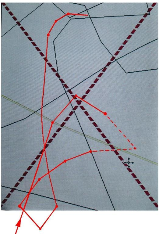
There was a loss of satellite reception of the GPS during the first turn to the right. This is shown on the picture by a dashed red line.
