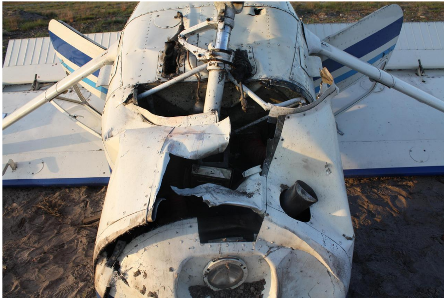
Figure 16: Wreckage with view on broken nose landing gear strut.
