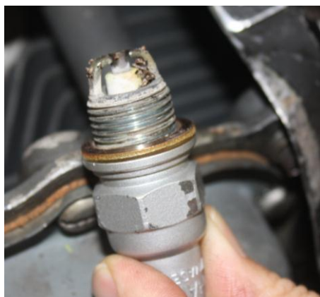
Figure 18: Spark plug with combustion deposit
