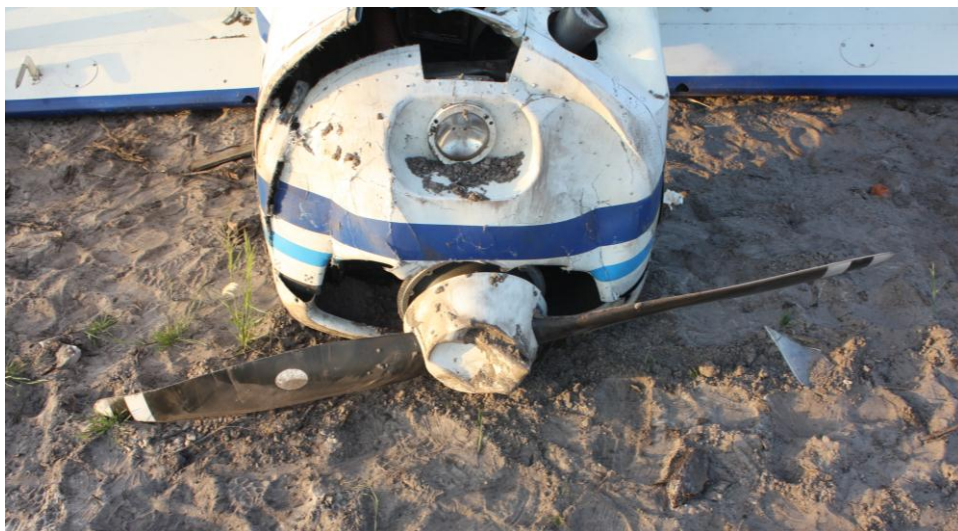
Figure 17: Propeller blades slightly damaged
