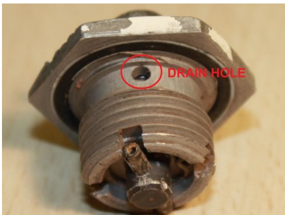
Figure 11: Drain hole in the drain chamber
