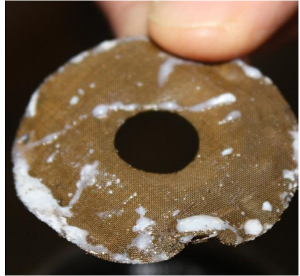
Figure 10: gascolator screen filter
