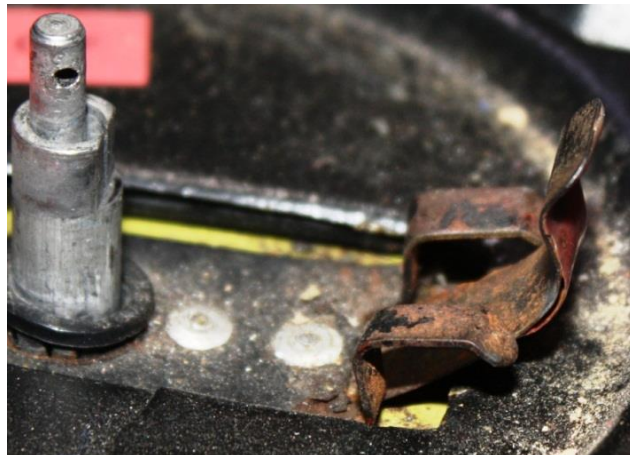
Figure 7: fuel selector Valve safeguard
