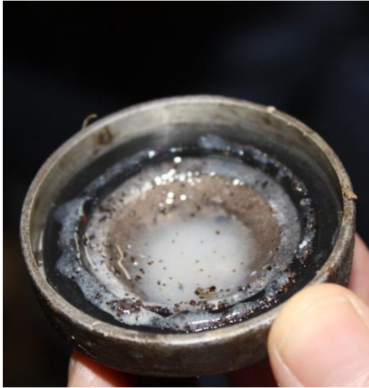
Figure 9: Bottom cover of the gascolator
