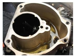
The carburettor was carefully inspected in order to find the reason of the low quantity of fuel found in the bowl. The "Nose down" position of the airframe after the accident could not explain such a significant loss of fuel. The float and the float valve and seat did not show any anomaly. The fuel inlet strainer was clean.
