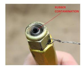
The contaminated flexible line was inspected again and it was determined unlikely that the rubber shaving contamination could have moved and fully obstructed the fuel flow.
