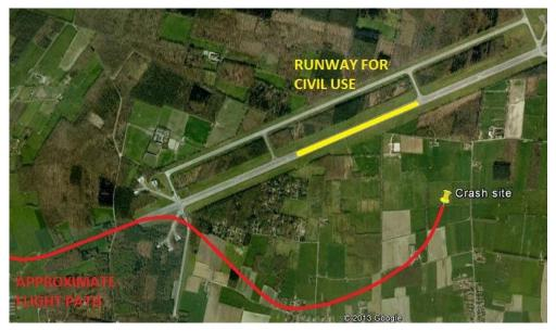
The flight path was reconstructed based on the declaration of the pilot. Considering he had missed the approach, the pilot decided to stop the exercise when he was flying at around 1000 ft above the threshold of the Air Defence runway.
