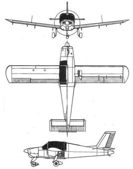
**General characteristics**: Length: 7.25 m, Span: 9.74 m, Max. take-off weight: 770 kg, Power plant: Continental O-200-A piston engine, Fuel tank total capacity: 104 liters (52 liters in each wing). **Performance**: Never exceed speed: 250 km/h, Cruise speed: 200 km/h, Speed range flaps down: 75 – 120 km/h, Speed range flaps up: 85 – 200 km/h, Best glide speed: 130 km/h with flaps and slats retracted, Lift to Drag ratio: more than 10.
