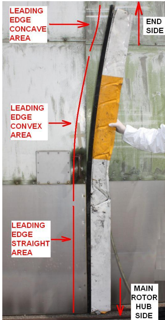
Figure 9: Separated 2,3m long section of MR blade.
