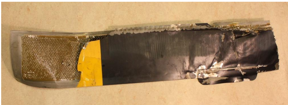
Figure 13: Separated 0,75m section of MR blade without beam/leading edge.
