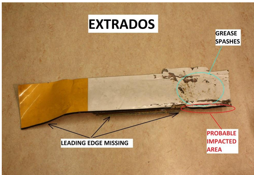
Figure 20: Extrados of 0,67m end section.
