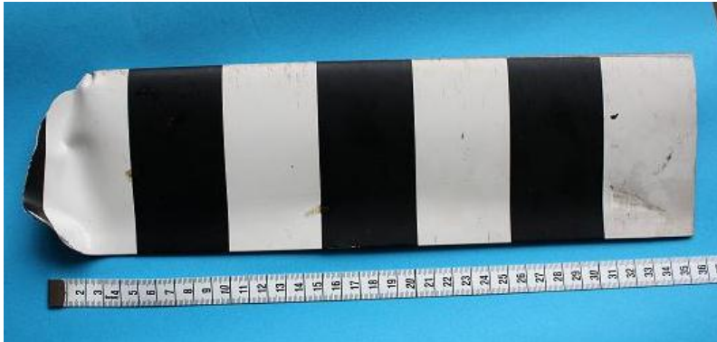
Figure 10: Separated tail rotor blade.
