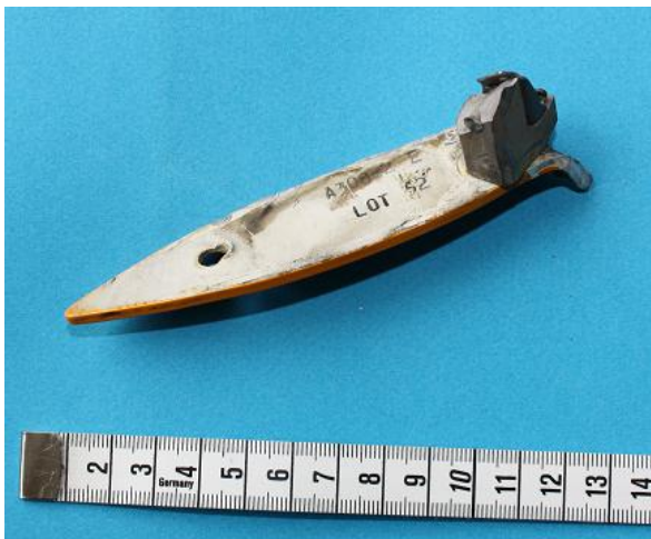
Figure 11: Separated main rotor tip end.
