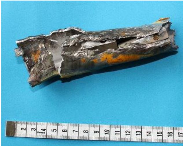
Figure 12: Separated main rotor beam/leading edge end.
