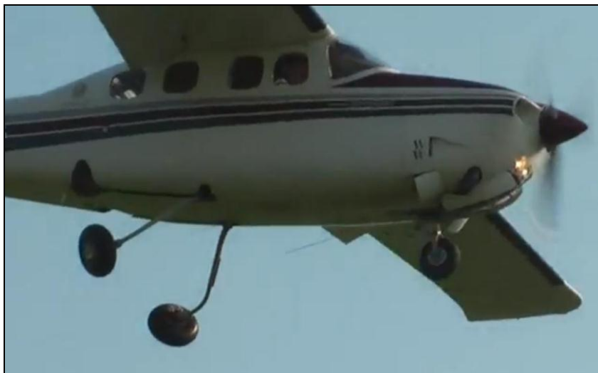
Figure 1: Image from the video showing that main landing gear was not fully extended
