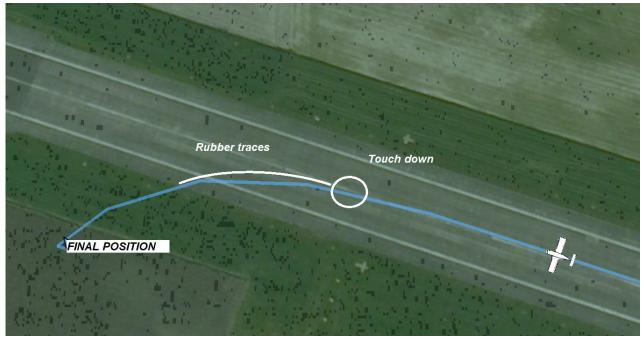
Figure 2: touchdown and deviation on RWY 29 at EBFN
