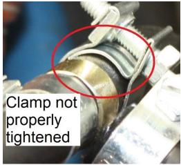
Figure 9: gap between the clamp and the rubber pipe.
