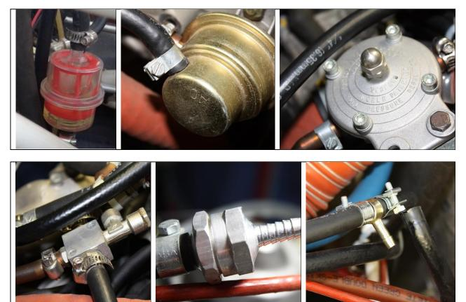
Figure 10: pictures showing different clamp and connection types.
