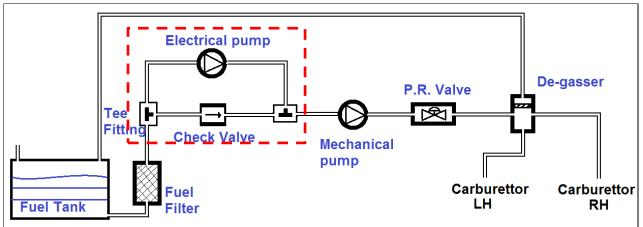
Figure 4: Fuel system after modification
