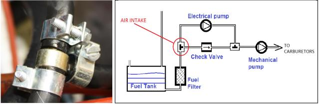
Figure 7: tee fitting connection showing a Figure 8: Position of the leaking tee fitting connection sweaty leak
