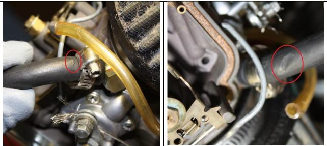
Figure 11: cracks in a rubber line
