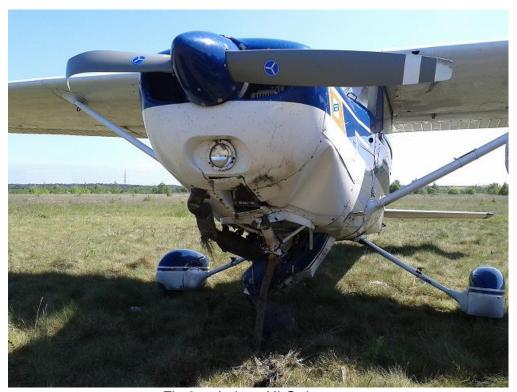
Fig.2 airplane NLG damage
