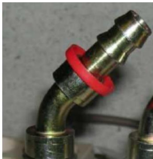
Figure 9: Picture of a connector before installation of the rubber pipe
