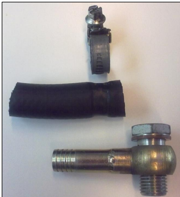
Figure 7: Picture of the failed oil cooler connection
