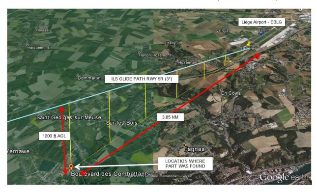
Figure 1: A scheme of the ILS approach glide path of runway 05R showing the location where the part was found
