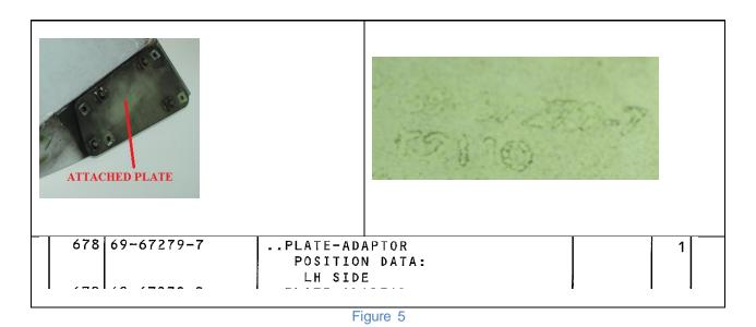
The fasteners are missing, although the remains of one is still lodged between the plate and the main body.
