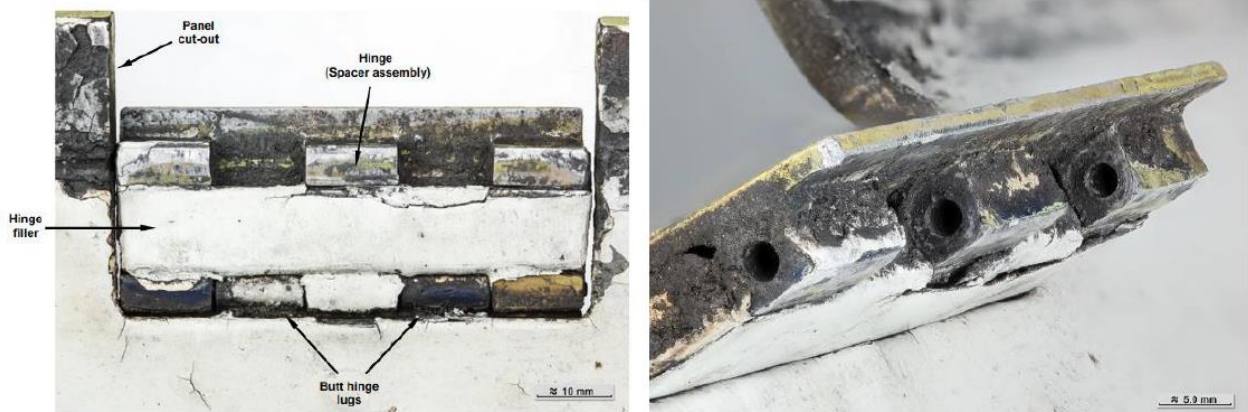
General view of forward hinge assembly
