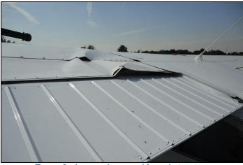
Figure 3: damaged upper skin and structure
