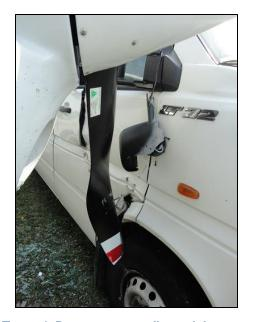
Figure 4: Damage to propeller and the van
