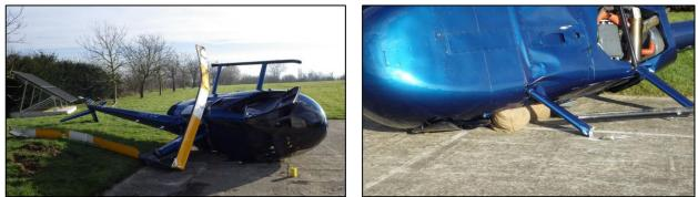
Figure 1: pictures showing damage to the helicopter and the burlap bag involved
