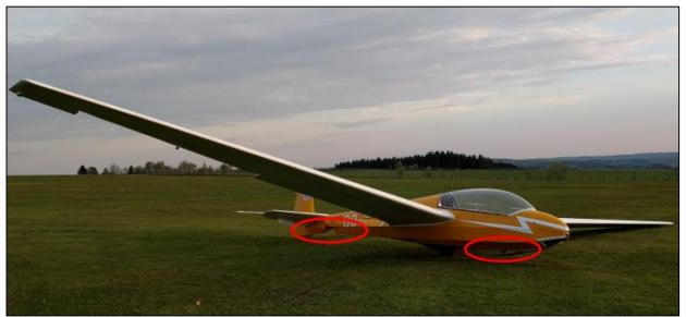
Figure 1: areas showing visible structural damages
