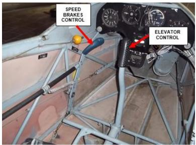
Figure 7: Elevator and airbrakes controls
