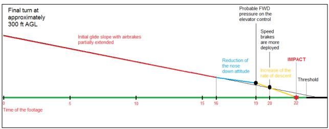
Figure 13: Approximate (not on scale) view of the glide path
