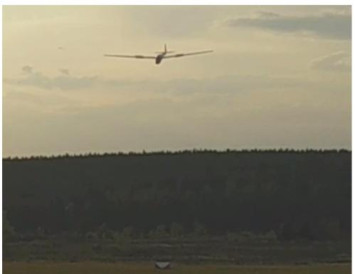
Figure 9: After 19 seconds, the nose down attitude is noticeably increased. No visible modification of the airbrakes' position.
