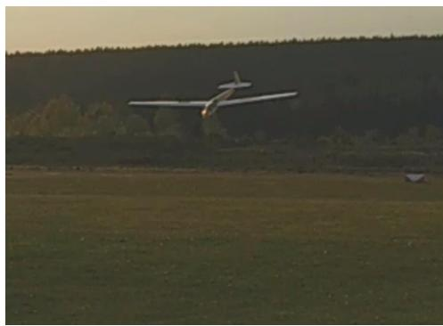
Figure 12: After 22 seconds, last useable picture in flight: the pitch down attitude seems to be again increased for a fraction of a second just before impact. No visible attempt to flare.
