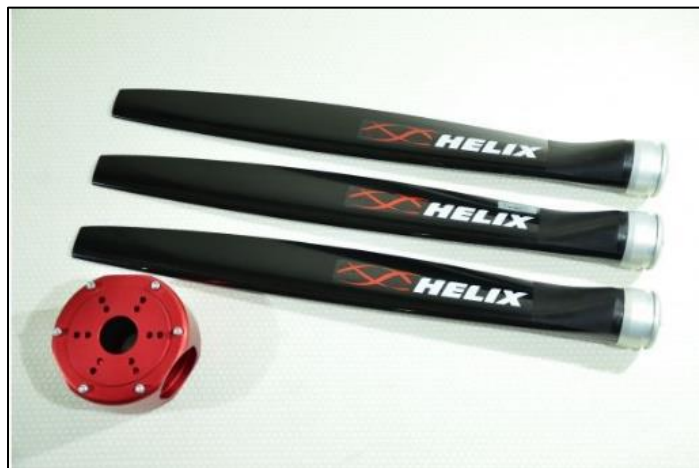
Figure 6 : View of H60V 1,75m R-TS-3 shortened 1,60m
