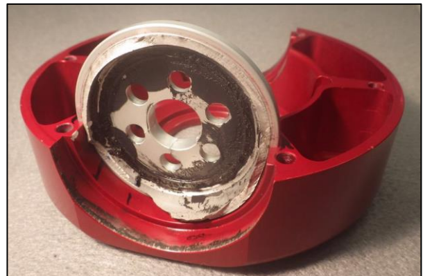
Figure 11 : broken part of the blade root left in the hub
