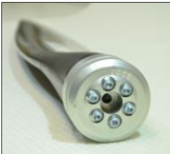
Figure 7: Aluminium root of the blade
