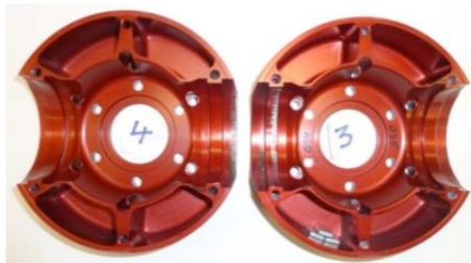
Figure 16: view on both hub halves, showing sliding grooves created by failure of propeller blade 2; no significant traces have been observed on the location for undamaged propeller blade 1
