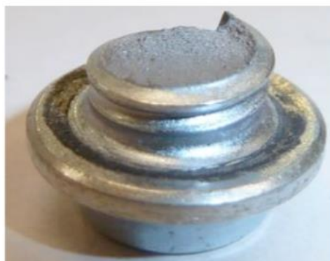
Figure 14: ductile fracture surface of bolt No.3
