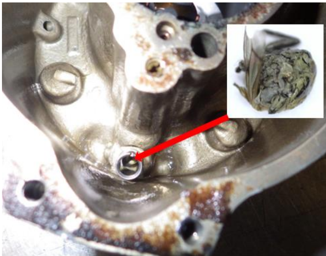
Figure 4 Location of the fly in the sleeve of the metering valve.
