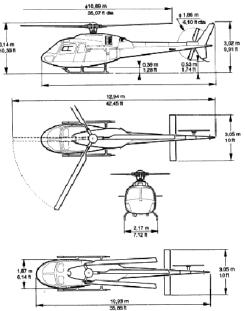
Figure 4:helicopter lay-out and dimensions
