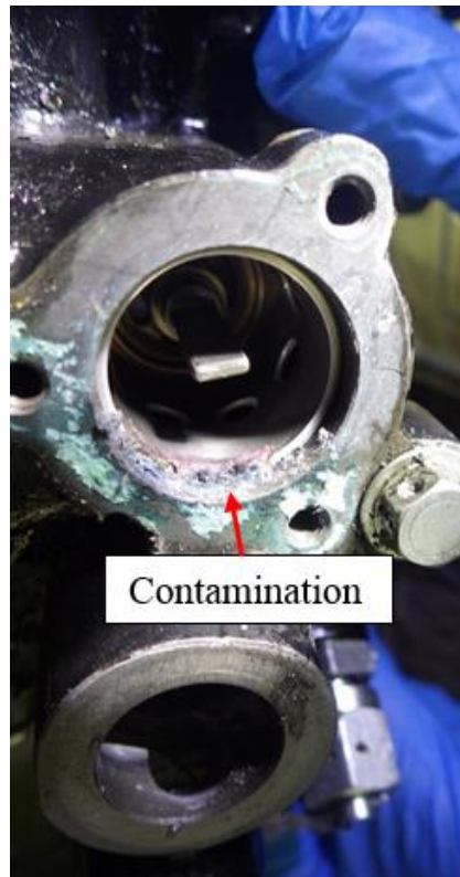
Figure 27: Upper bore: metering valve chamber.
