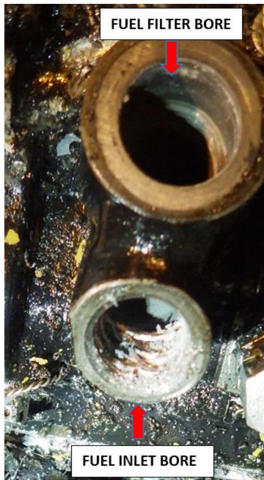
Figure 23: fuel inlet bore just after removal of the elbow fitting
