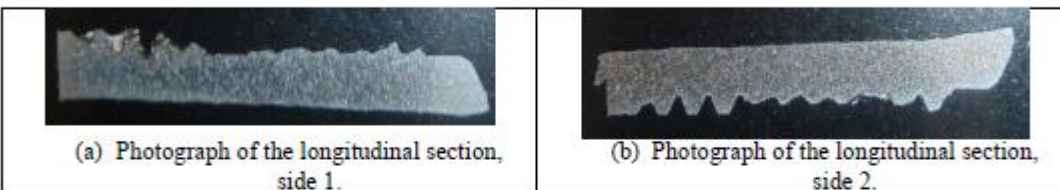
Figure 10: Photographs of the cut out section of the fuel inlet bore, showing signs of wear and/or corrosion.
