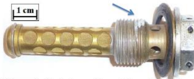
Figure 16: Photograph of the fuel screen filter, with the particles visible on the thread.
