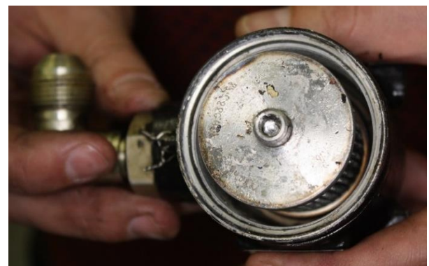
Figure 26: Fine filter underside, as seen just after removal of the cover
