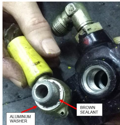
Figure 17: Fine fuel filter after the outlet fuel line removal.
