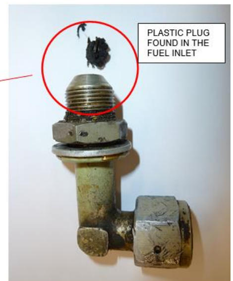
Figure 10: Fuel inlet elbow of the fuel shut off valve
