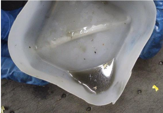
Figure 15: Dirty water from the compensation tank.
