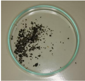
Figure 11: Particles found inside the shut off valve
