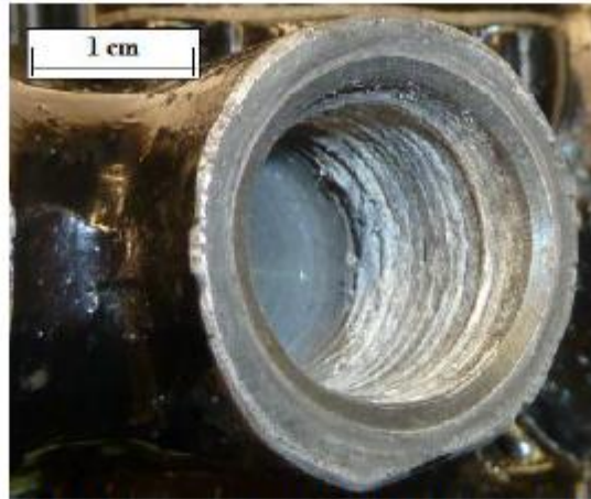
Figure 5: Alleged two-component paste on the fillet of the fuel inlet bore
