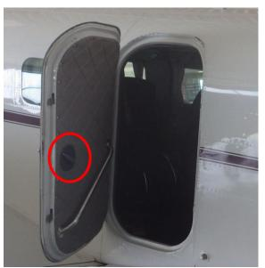
Figure 12: Position of the latch to open the back door
