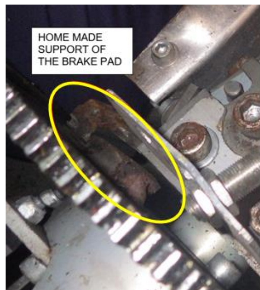
Figure 13: Bad welding of a support for a non-genuine rotor brake pad.
