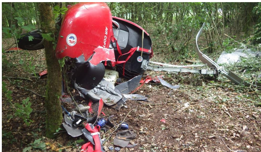
Figure 3: The left side of the cabin was completely destroyed.
