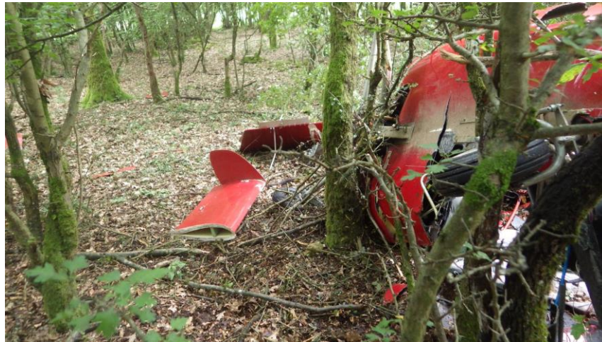
Figure 4: Scattered tail parts in relation to the belly of the cabin.
