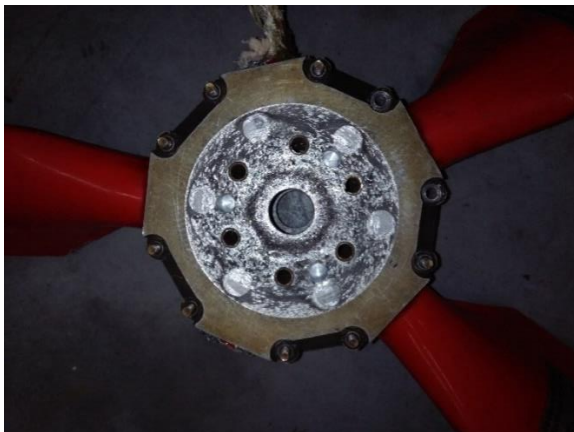
Figure 15: propeller hub damaged by severe fretting
