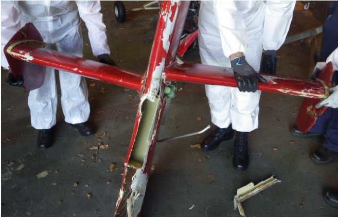
Figure 9: Reconstruction of the tail section.
