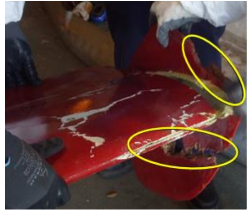
Figure 10: Damage compatible with rotor blade impacts.
