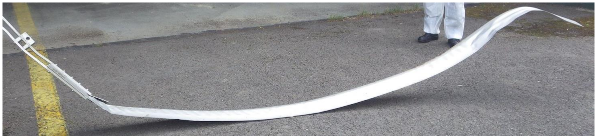
Figure 5: One rotor blade (with the hub bar still attached) featuring a S shape
