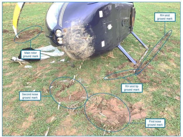
Figure 11 Detail of the nose and RH skid tip ground marks
