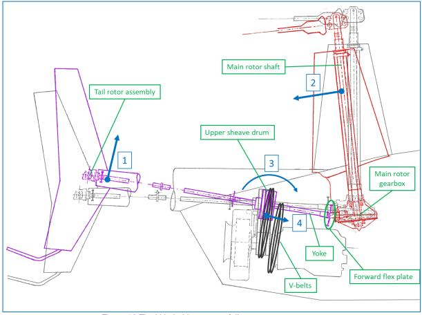
Figure 18 The V-belt drive system failure sequence
