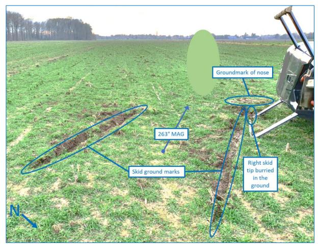
Figure 10 Direction of the helicopter and ground marks of skids and nose
