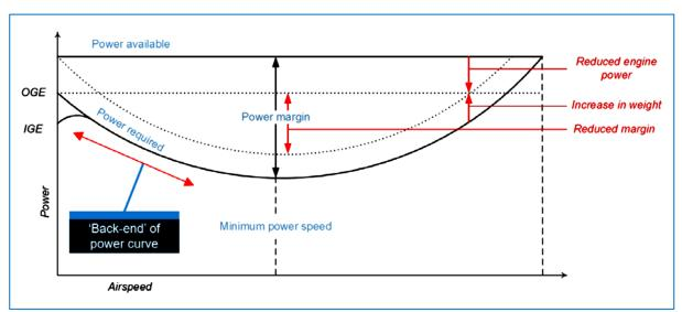
Figure 17 Typical power curve of a helicopter (source: ATSB)
