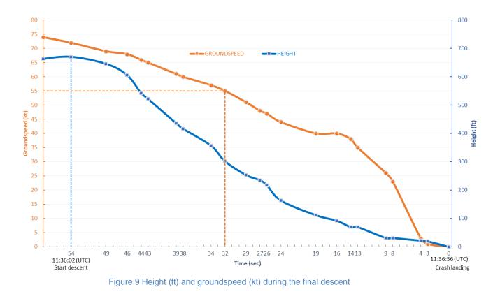
The Rate of Descend (RoD) and track were both derived from the flight data:
