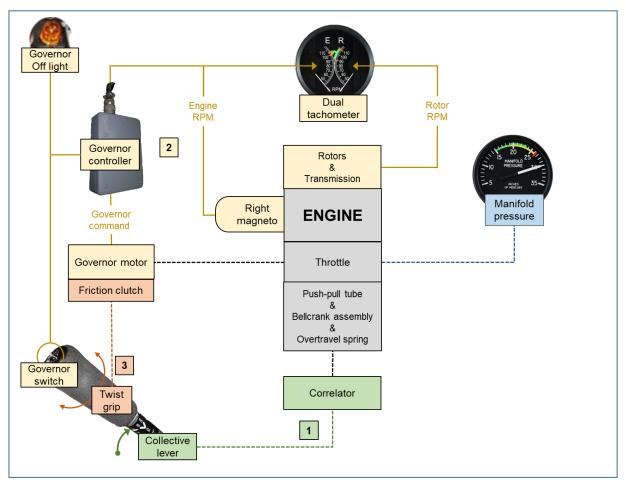
Figure 5 Schematic presentation of the engine throttle control
