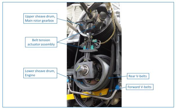
Figure 13 Damage on the drive belt system
