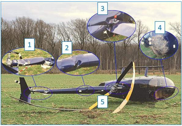
Figure 12 Aircraft damage
