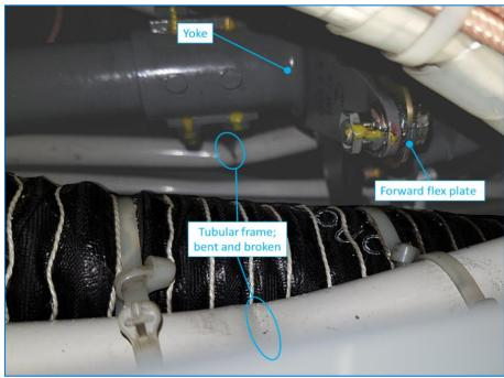
Figure 15 Damage on the tubular frame structure
