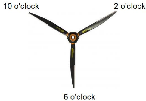
Figure 18: Blade position convention (view from the front of the aircraft)
