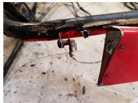
Figure 12: Trim tab broken hinge
