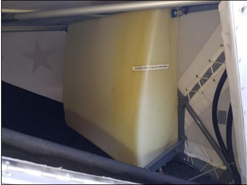
Figure 5 : Auxiliary Fuel Tank (fuselage - behind the cockpit – another Rans Coyote aircraft)
