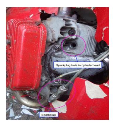
At first inspection of the wreckage, a sparkplug was found out of its hole in the cylinder head.
