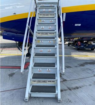
Figure 6 : front view of the Boeing 737-800 airstairs
